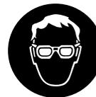
To reduce the risk of eye injuries, wear close-fitting safety glasses in accordance with European Standard EN 166. Make sure the safety glasses are a snug fit.
